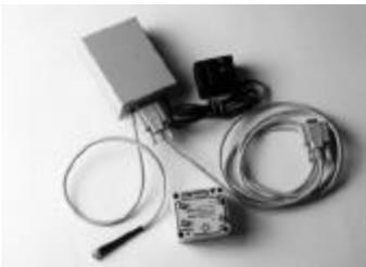
This is a standard configuration for the MOD-1A loggers. The wall-mount power supply would be plugged into a wall socket and the small cord would be plugged into the SIA module. The 9-pin connector cable would connect the SIA module to a COMM Port on the PC, and the remaining cable would plug into the I/O socket on the logger module.
